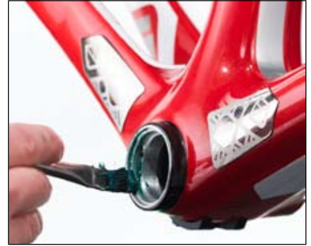
Figure 21. Greasing the bearing and the frame saddle
